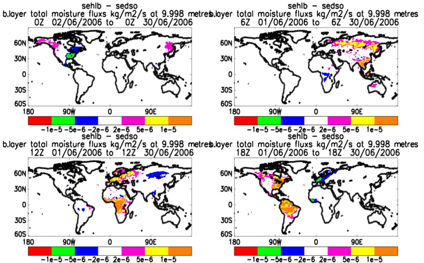
Figure 19: Impact of the two-stream multi-layer canopy radiation scheme on surface evaporation.
