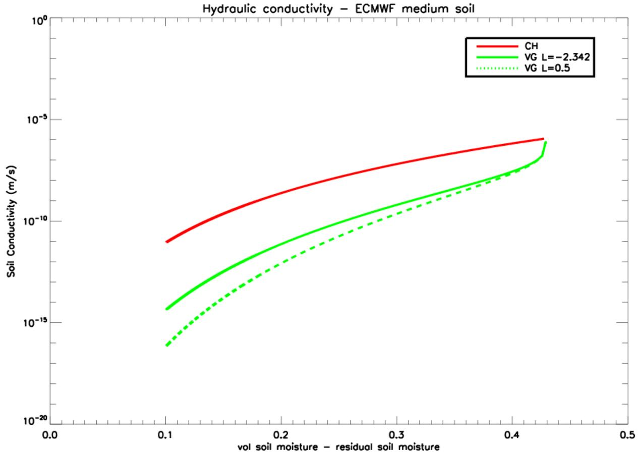
Figure 23: Example comparing the relationship between  $\theta - \theta_r$  and soil hydraulic conductivity for the VG (green curves) and CH (red curve) parametrisations. The soil parameter values used are the same as in Figure 22. The solid green curve uses the ECMWF value that  $L = -2.342$  and the dashed green curve assumes that  $L = 0.5$ . The saturated hydraulic conductivity  $K_s = 1.16 \times 10^{-6}$  m/s.
