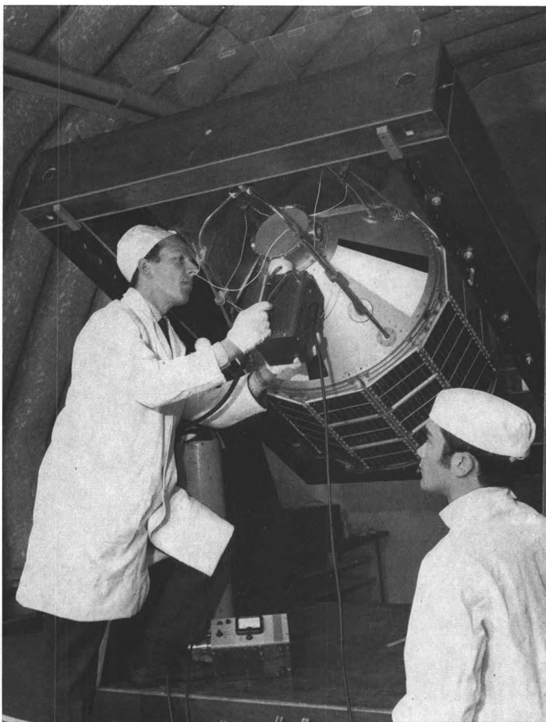
Carrying out final checks on the Meteorological Office Molecular Oxygen Experiment on the satellite UK-3.
