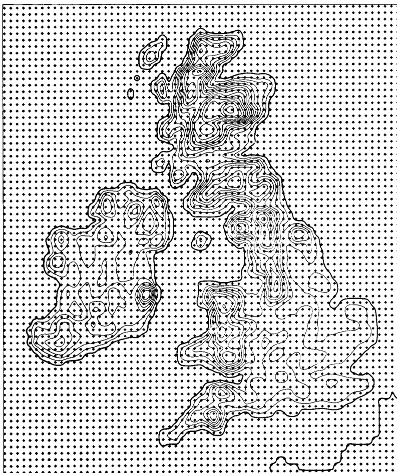
Figure 1. Model domain and orography. The grid points have a 15 km spacing and the contour interval is 50 m. The bold contour is at zero metres and indicates the model coastline.
