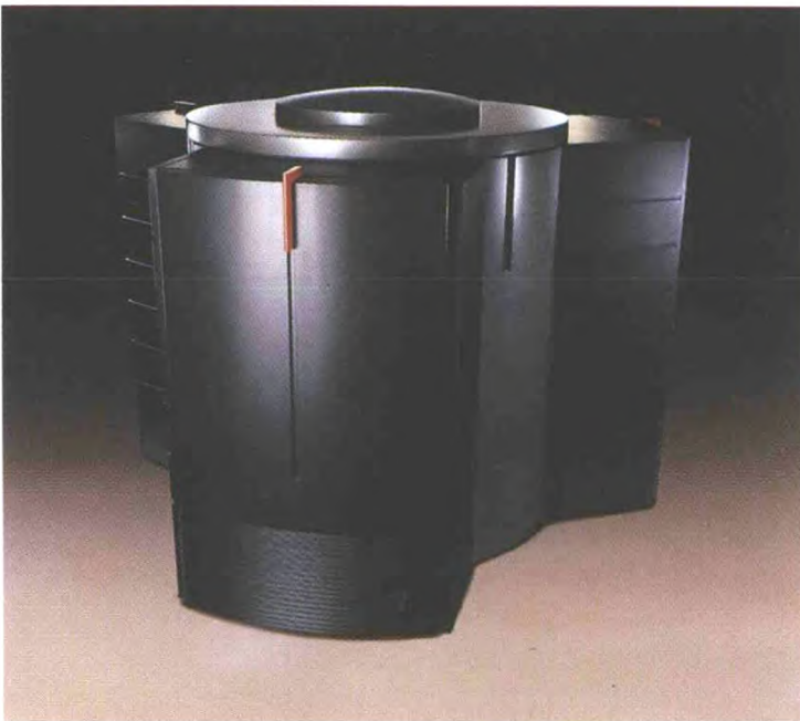
CRAY C916, the model that is installed at the Meteorological Office. The system has 16 processors and has a peak performance rate of 16 GFlops (16 billion floating point operations per second). One floating point operation involves adding, subtracting, dividing or multiplying two numbers to an accuracy of 14 decimal places.
