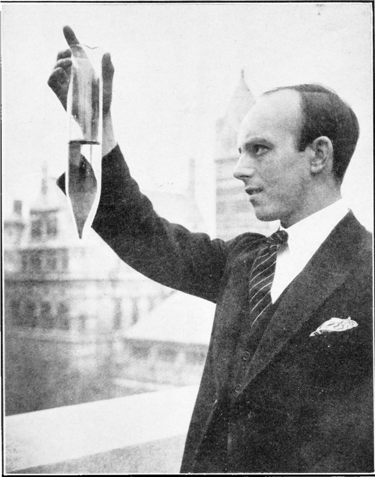
FIG. II.—THE NEW TAPERED RAIN MEASURE IN USE.
