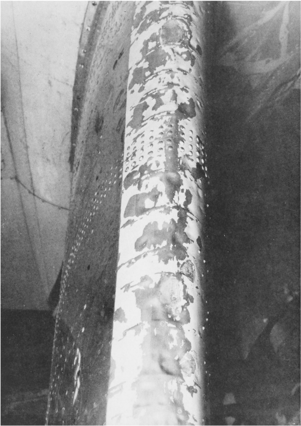
Close-up of leading edge of starboard tailplane HAIL DAMAGE TO A BRITISH EUROPEAN AIRWAYS VISCOUNT (see p. 80)
