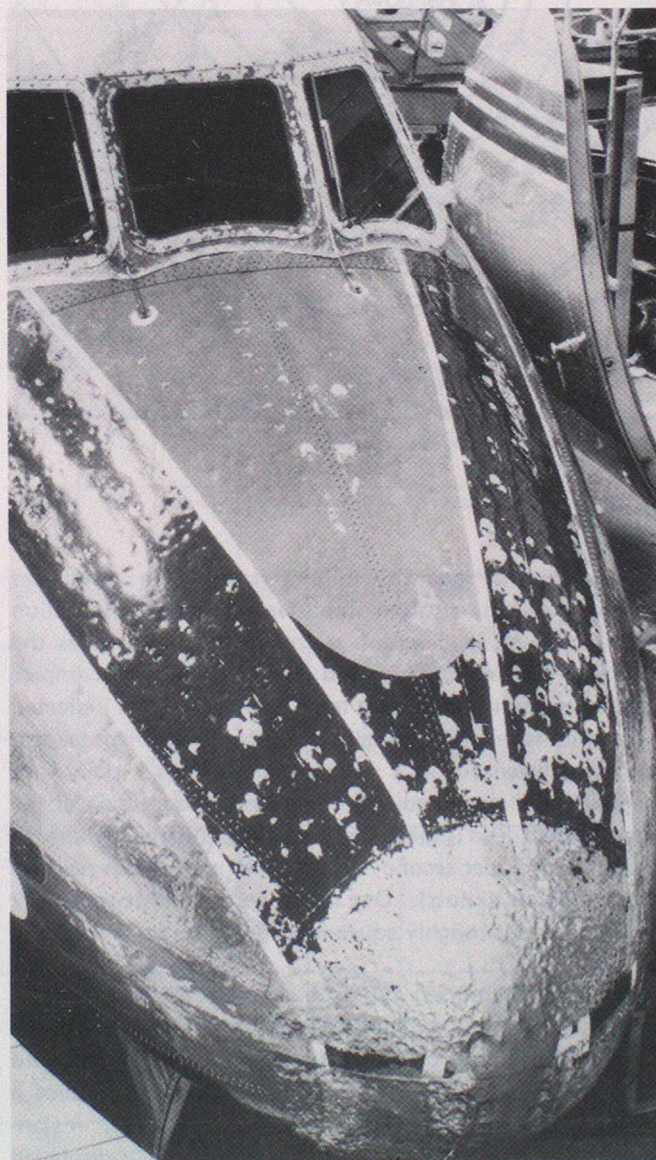
Hail damage to nose of aircraft
