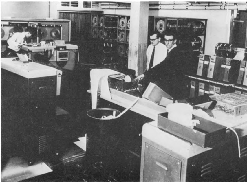
Plate V. KDF9 computer Comet showing console, magnetic tape decks and paper-tape readers.
