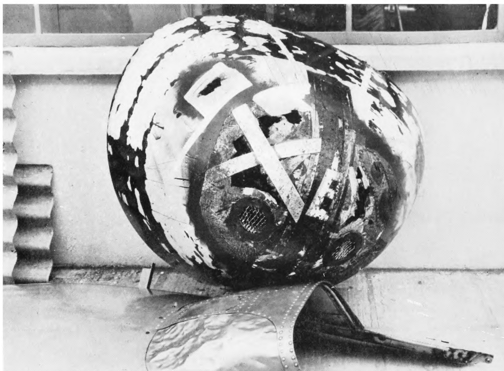
DAMAGE TO NOSE OF AIRCRAFT
