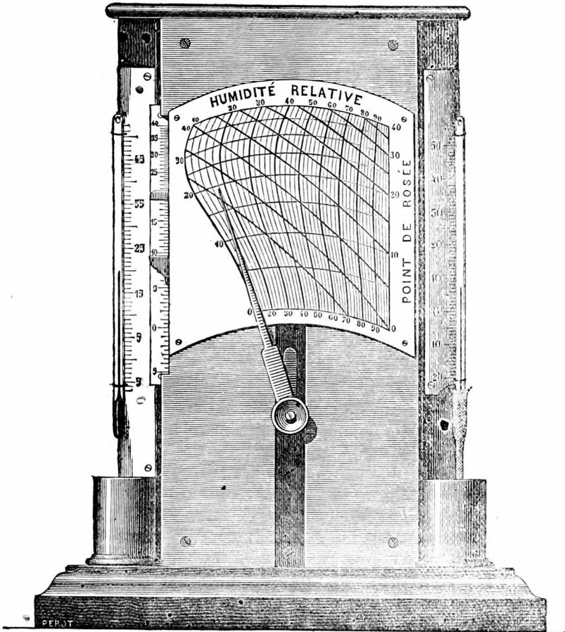
indices travelling upon it. In the middle there is a knob with a long pointer attached to it, which can be raised or lowered, and also turned round.
