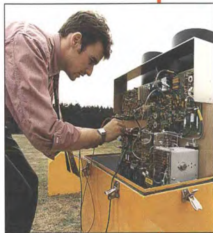
Technicians regularly service observational equipment, in this case a Laser Cloud-base Recorder
