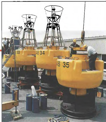
Buoys are built, tested and dismantled prior to deployment. These are now in use in the Atlantic, 200 miles off the west coast of Ireland
