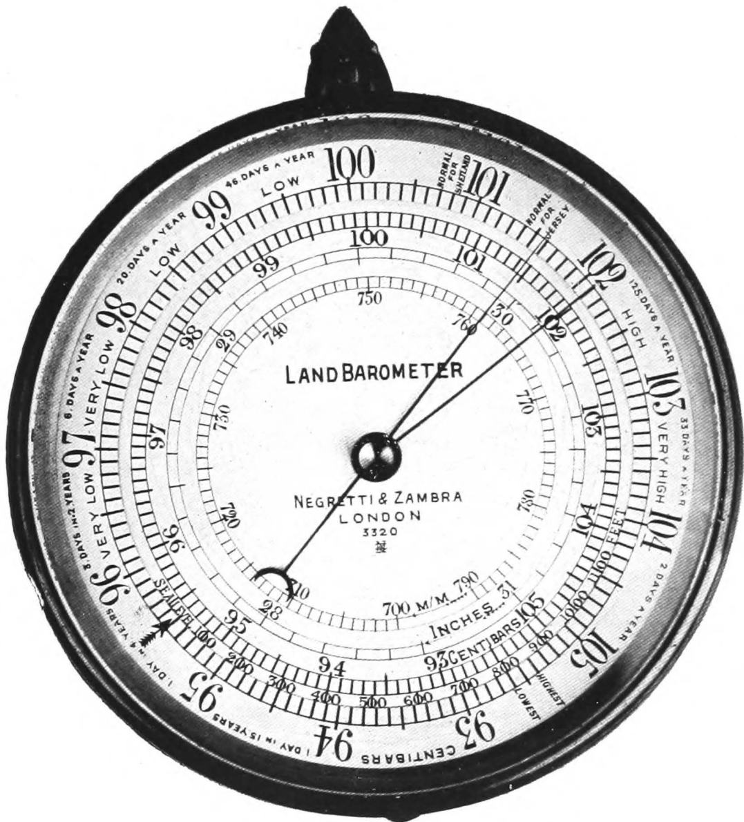
FIG. 1. LAND BAROMETER. (See pp. 49, 65.)
