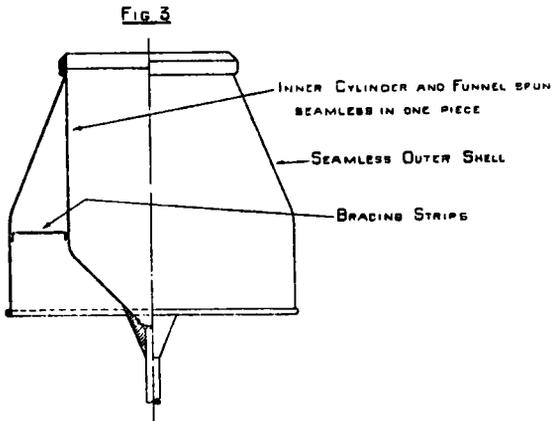
tubing for the construction of rain-gauges. By this means, all vertical seams can be avoided, not only in the funnel, but in the outer vessel and the inner can. There would remain, however, the seam B in Fig. 1, although the seam C could be eliminated by spinning
