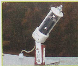
Kipp and Zonen automated sunshine recorder
