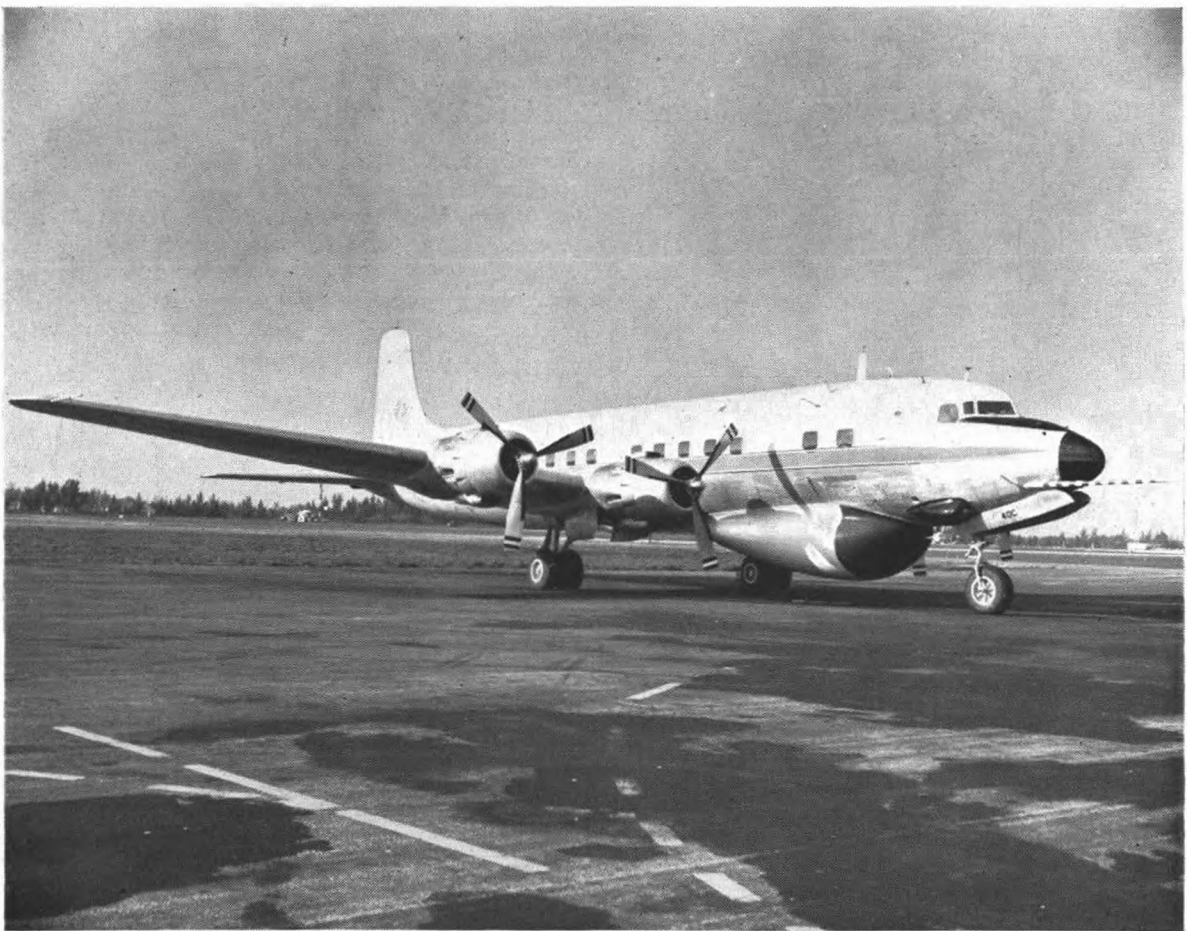
1. DC-6A of the U.S. Weather Bureau's Research Flight Facility. The gust probe protrudes in front of the nose; the small blister rearward of the nose wheel houses a 16 mm. cloud movie camera, the large blister houses an 8 ft. search radar antenna, doppler antenna and radio altimeter antenna; various protrusions on the top of the fuselage, house temperature and liquid water measuring devices. (See page 74.)
