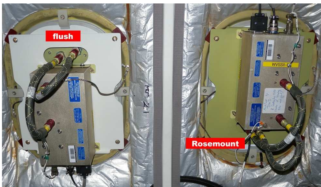
Plate 1. Installation of WVSS-II sensors on FAAM aircraft.
