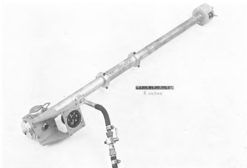
PLATE III(a)—IMPACTOR USED FOR SPORE COLLECTION BY AIRCRAFT
