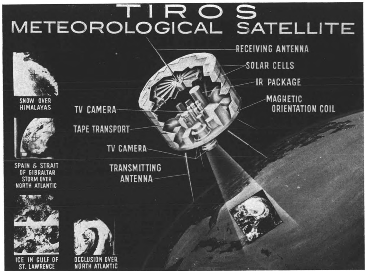
Fig. 1. This diagram shows the meteorological sensors of TIROS. The IR (Infra-Red) package is a multiphase radiometer. The photographs give an idea of the area that can be seen in a single photograph, and the uses of the photographs. Directly beneath the TIROS is a picture of Hurricane 'Betsy' (July 1961). (See page 141.)
