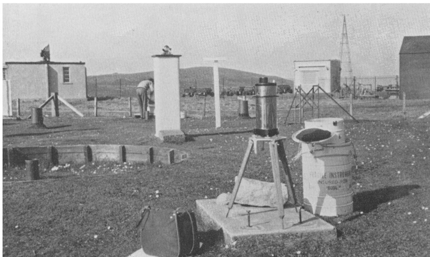
PLATE VI—GRAVIMETER SET UP TEMPORARILY IN THE INSTRUMENT ENCLOSURE IN 1961
