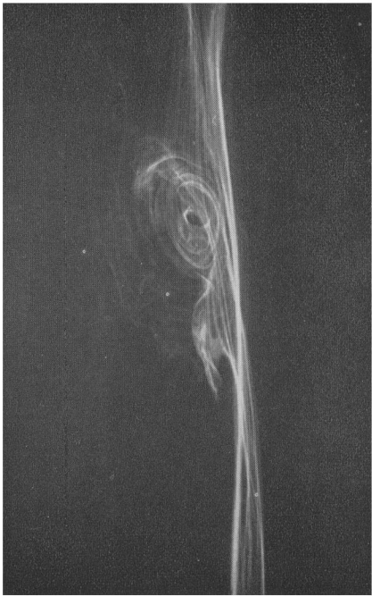
(c) End view of the breaker roll, with a secondary breaker.
