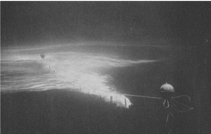
PLATE II—A HORIZONTAL ARRAY OF FLUORESCIN PACKETS INJECTS DYE INTO A THERMOCLINE SHEET, SHOWING THE LAMINAR FLOW Note the internal wave visible at the top of the picture.
