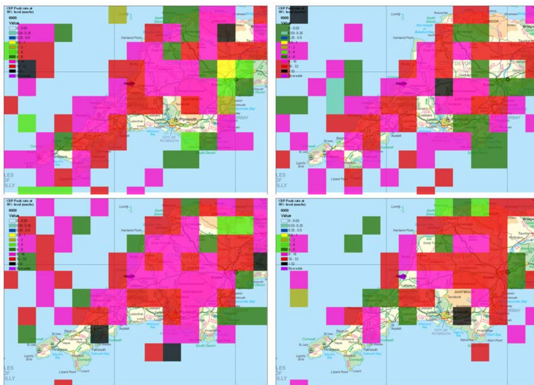
Figure 24 Peak convective rain rates for 1300, 1400, 1500, 1600UTC, diagnosed using the Convection Diagnosis Procedure (CDP) from the large scale conditions in the mesoscale model in 15km squares. Heavier values shown are black: >32mm/hr, red: >16mm/hr, pink: >8mm/hr, dark green: >4mm/hr.
