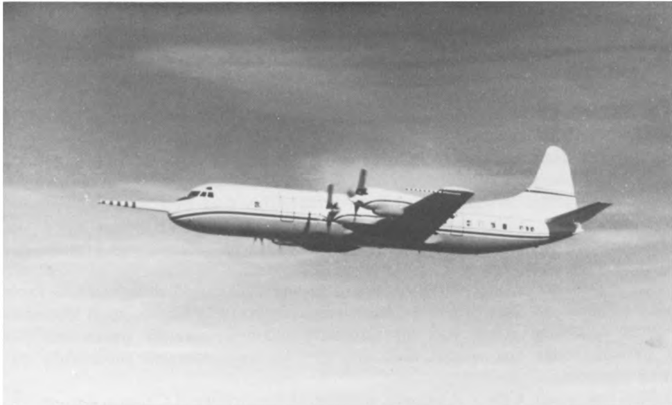
Figure 1. One of the highly instrumented long-range research aircraft participating in ALPEX. (USA Lockheed 'Electra'.)
