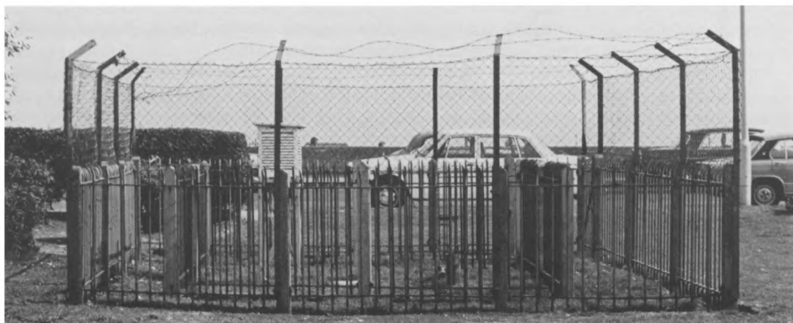
Figure 2. Auxiliary Reporting Station Gorleston. Instrument enclosure, with vandal-deterrent fence, at climatological site in public park.
