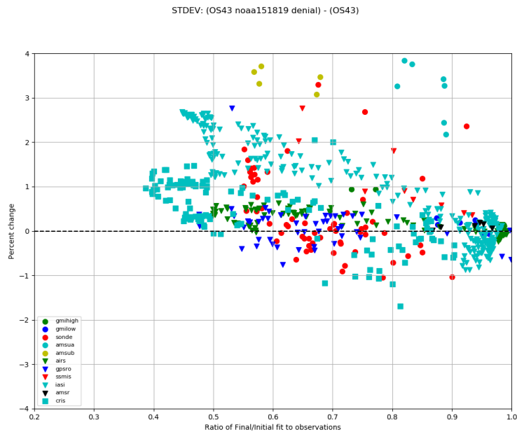
Figure 7. A summary of the percentage change in fit of O-B for each observation type between the NOAA-15, 18, 19 DDE and Control. Positive changes on the Y-axis signify degraded fit in the DDE. Each point from a given observation type represents a channel (for radiances) or layer (for radiosondes).
