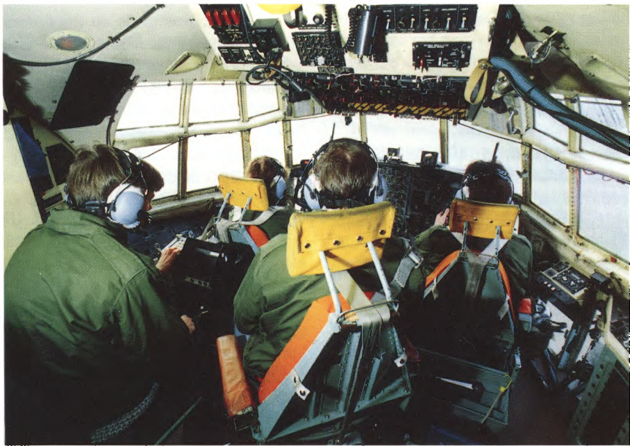
Figure 3. The operation of the meteorological sensors is coordinated by the Aircraft Scientist from the flight deck where he has a clear view through the aircraft window and can call up a graphical display of the real-time output of any sensor as required.
