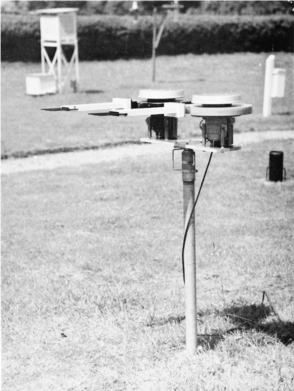
PLATE IV—VENTILATED NET FLUX RADIOMETER (see p. 287)
