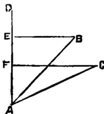
Let  $AB$ ,  $AC$ , represent the amounts received in gauges the mouths of which are at right angles to the path of the rain, at the heights of 1 ft. and 10 ft. respectively.  $AB$ ,  $AC$ , are therefore measures of the density of the rain at those heights.
