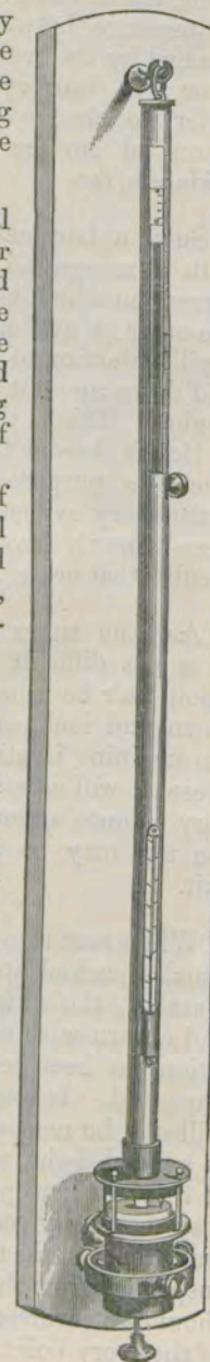
Barometers on Fortin's prin- ciple. Standard Barometer.
