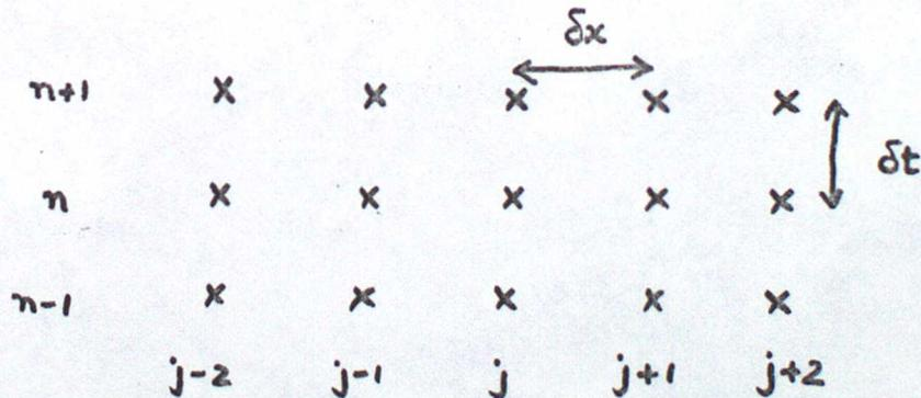
Figure 1 Finite difference grid for simple advection.
