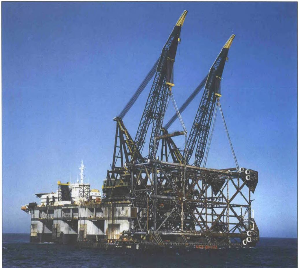
Heerema's giant crane DB102 lifting the Shell Gannet jacket from a barge
