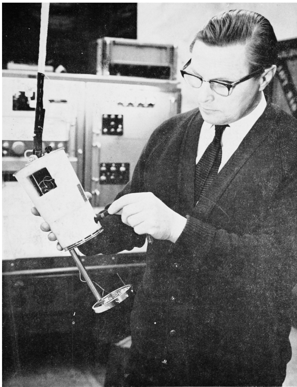
PLATE III—SETTING THE TRANSMITTER FREQUENCY OF THE ROCKETSONDE See page 327.
