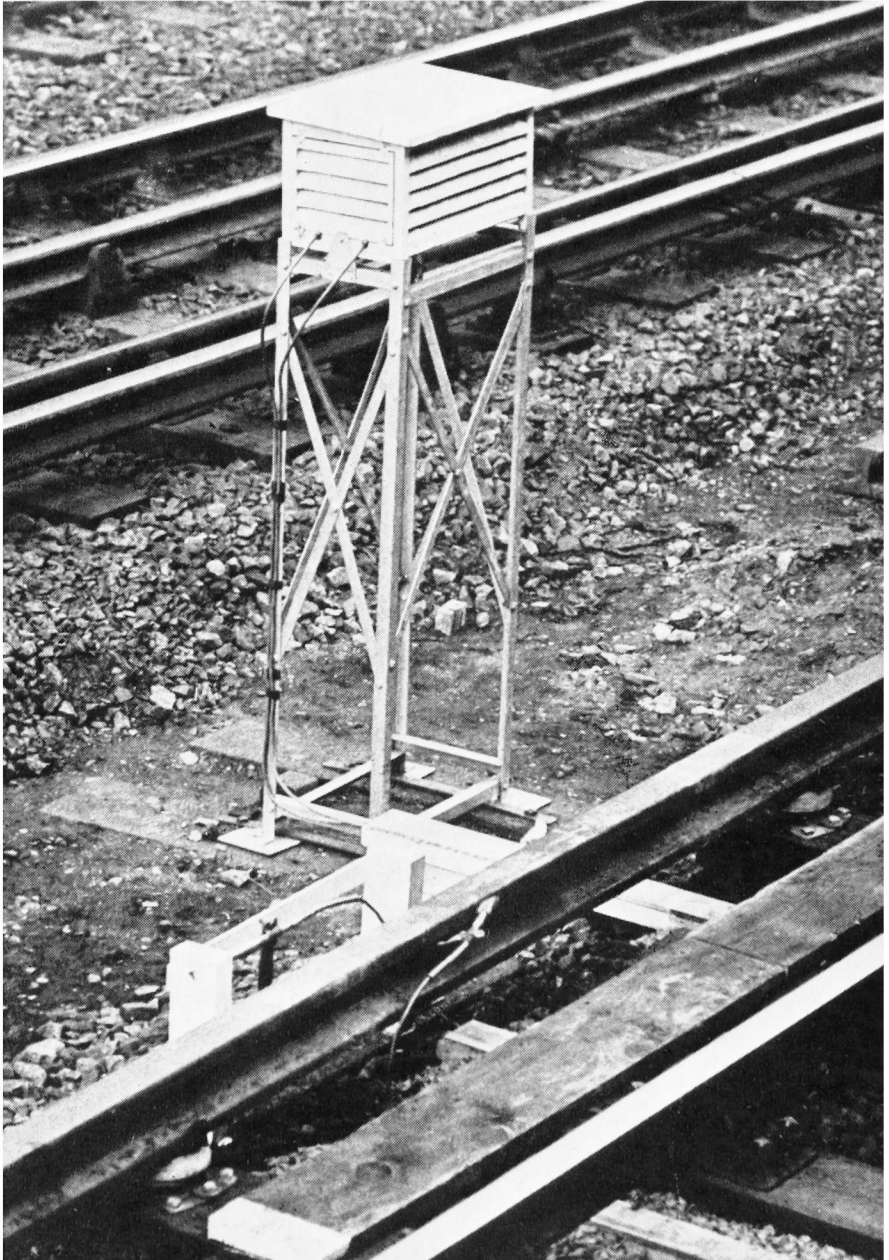
SCREEN HOUSING DISTANT-READING THERMOMETER BULBS
