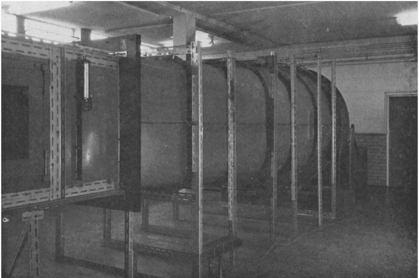
PLATE II—WIND-TUNNEL, SHOWING CONSTRUCTION OF EXPANDING SECTION BETWEEN WORKING SECTION AND FAN See page 146.
