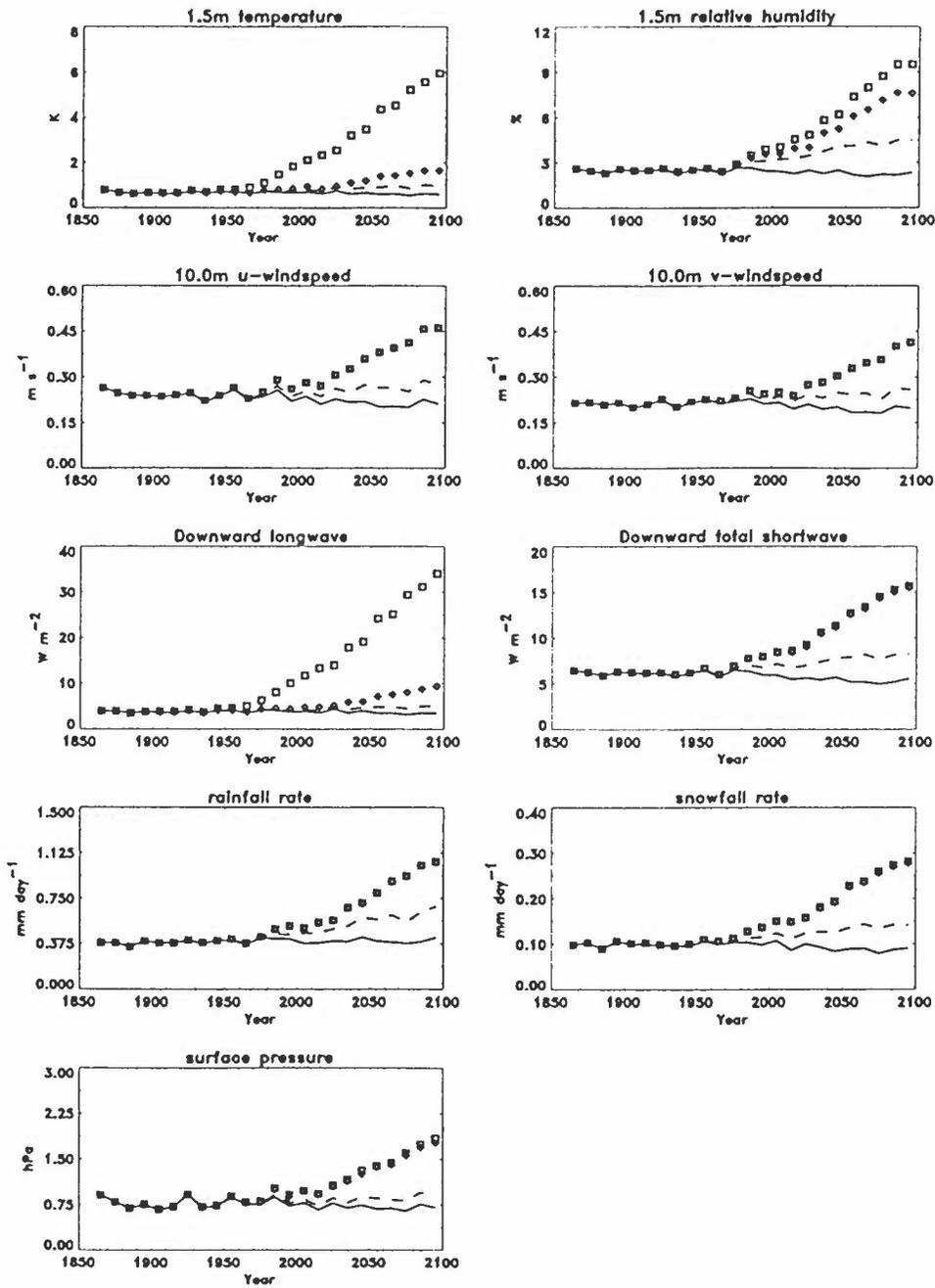
Figure 8: Values of  $\epsilon_V$  for each decade corresponding to predictions of the GHG GCM anomalies by the analogue model for each variable  $V$  (see individual plot titles) and using patterns derived from the GHG run (continuous lines) and the 2% run (dashed lines). Statistics  $\Delta V_{\sigma}(i)$  ( $\diamond$ ) and  $\Delta V_{TOT}$  ( $\square$ ) are also plotted.
