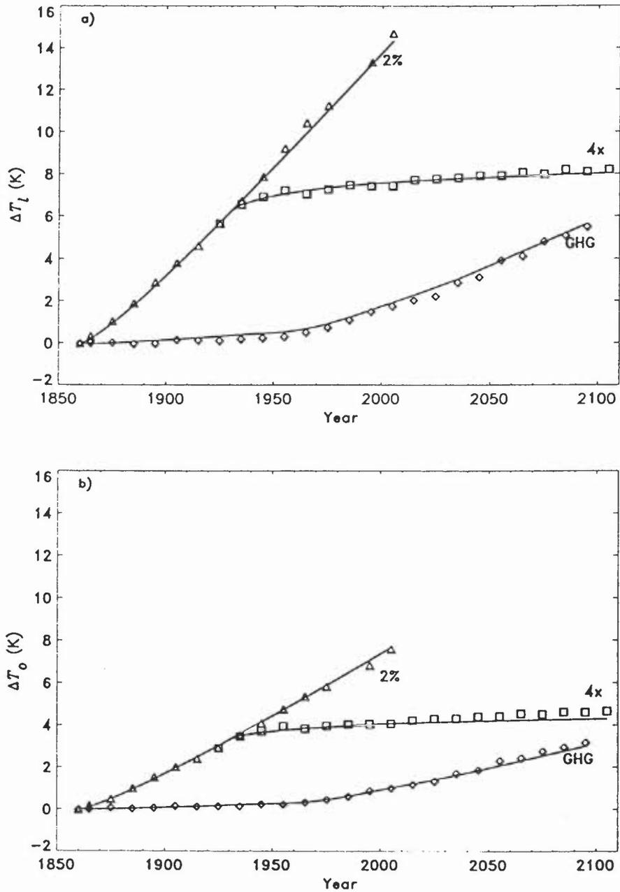
Figure 3: Two-box model predictions (continuous lines) of a) decadal mean land surface temperature and b) decadal mean ocean surface temperature, for radiative forcing scenarios appropriate to the 2%, 4x and GHG scenarios. Also plotted, for comparison, are the actual GCM decadal mean anomaly values for the ( $\square$ ) 2%, ( $\Delta$ ) 4x and ( $\diamond$ ) GHG GCM runs. The values plotted for 1860 are representative of long-term averages from a “pre-industrial” control run.
