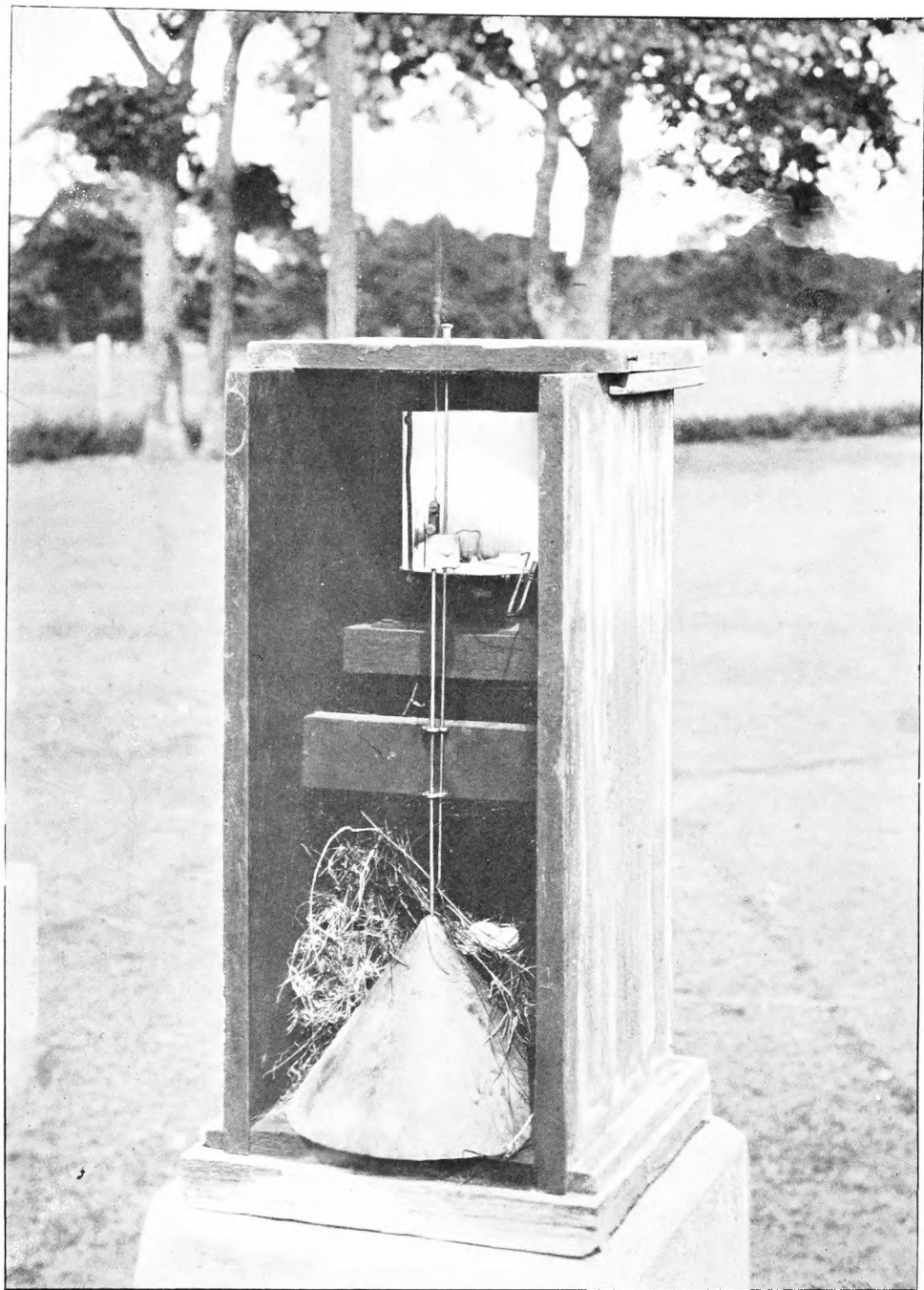
RECORDING ANEMOMETER AT COLOMBO, SHOWING BIRD'S NEST INSIDE.
