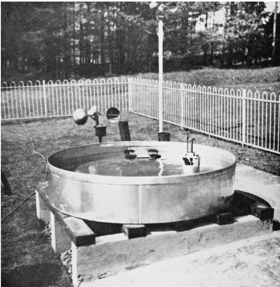
EVAPORATION PAN AT STOCKS RESERVOIR United States Weather Bureau class A type.
