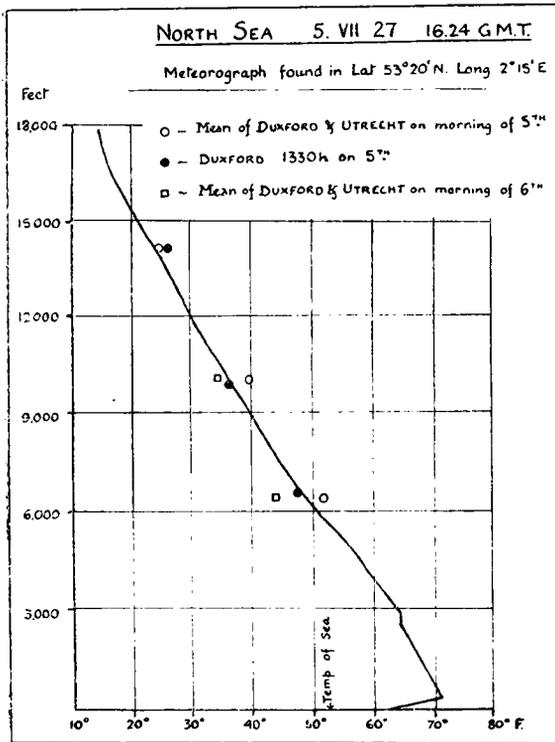
The record has been examined by Mr. L. H. G. Dines at Kew Observatory, and has been found to be quite legible. It gives a very remarkable surface temperature inversion, as shown on the accompanying diagram. Mr. Dines was able to trace on the record the point when the instrument went into the sea, where the pressure increased greatly; the temperature recorded at this point was  $53^\circ F.$ , and the temperature of the sea taken on board H. M. S. *Fitzroy*
