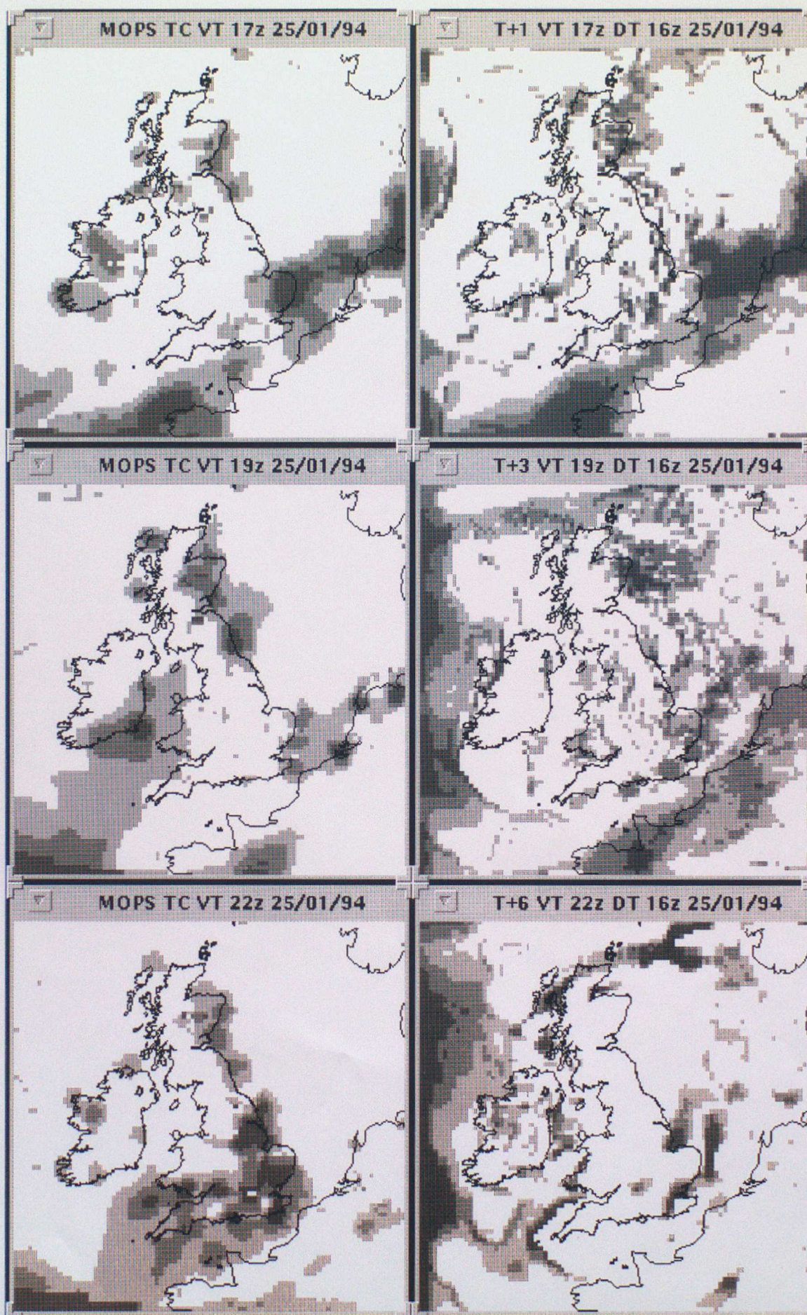
Figure 12. MOPS analyses and corresponding merged cloud amount forecast for total cloud at T+1, T+3 and T+6 from data time 25/01/94 1600 UTC. White = 6/8 - 8/8, light grey 4/8 - <6/8, grey 2/8 - <4/8 and dark grey 0 - <2/8 cover.
