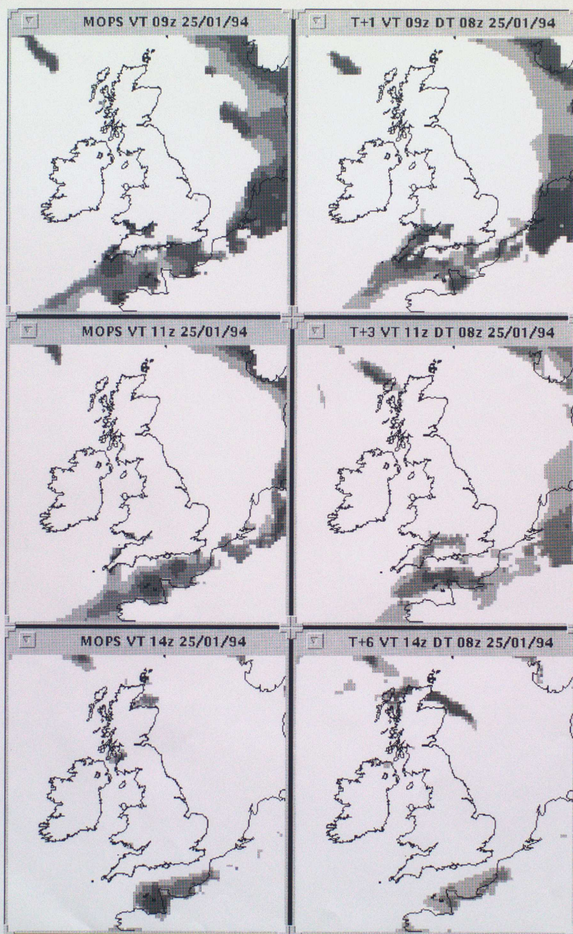
Figure 10. MOPS analyses and corresponding merged cloud amount forecast for low cloud at T+1, T+3 and T+6 from data time 25/01/94 0800 UTC. White = 0 - 2/8, light grey >2/8 - 4/8, grey >4/8 - 6/8 and dark grey >6/8 cover.
