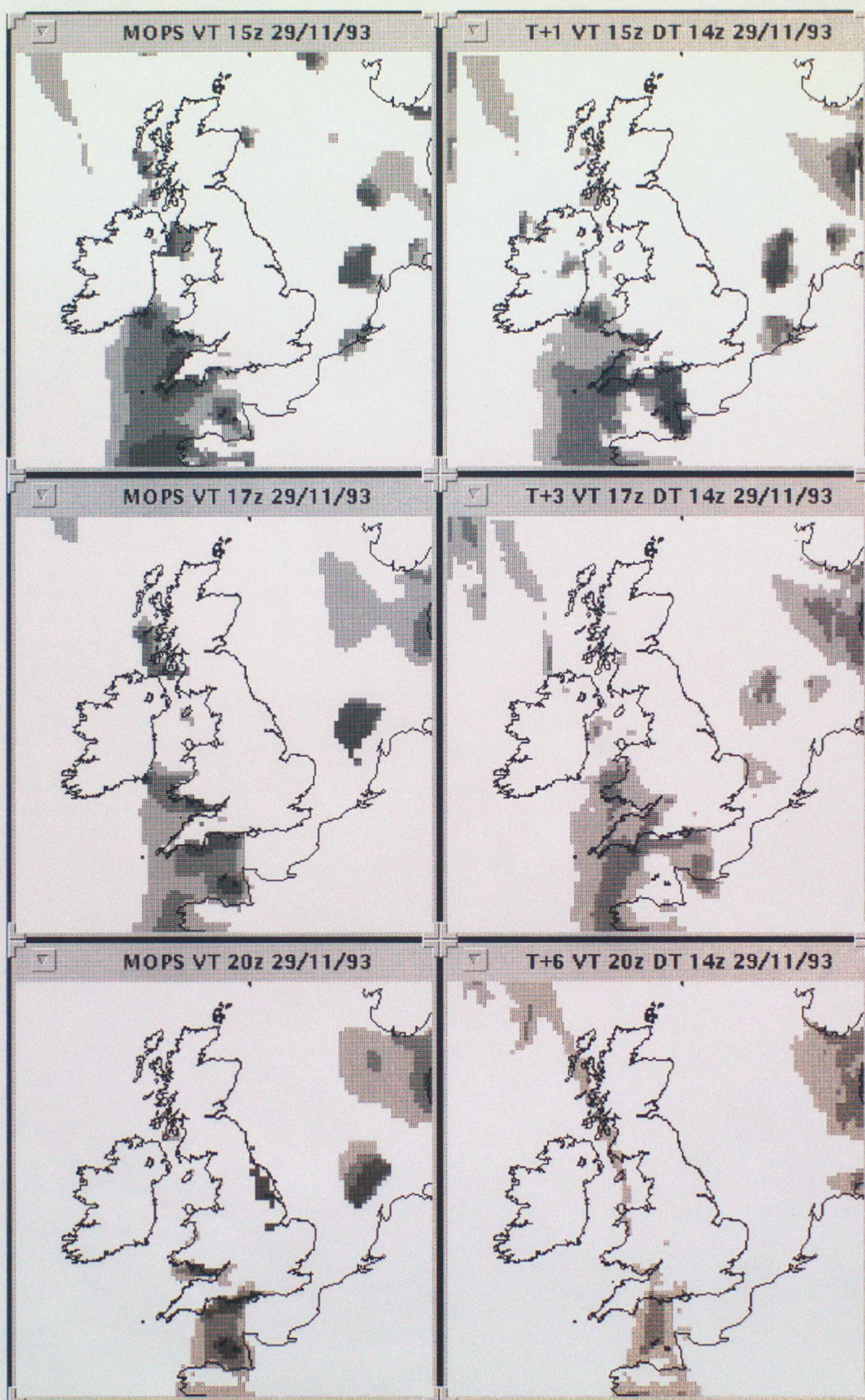
Figure 5. MOPS analyses and corresponding merged cloud amount forecast for low cloud at T+1, T+3 and T+6 from data time 29/11/93 1400 UTC. White = 0 - 2/8, light grey >2/8 - 4/8, grey >4/8 - 6/8 and dark grey >6/8 cover.
