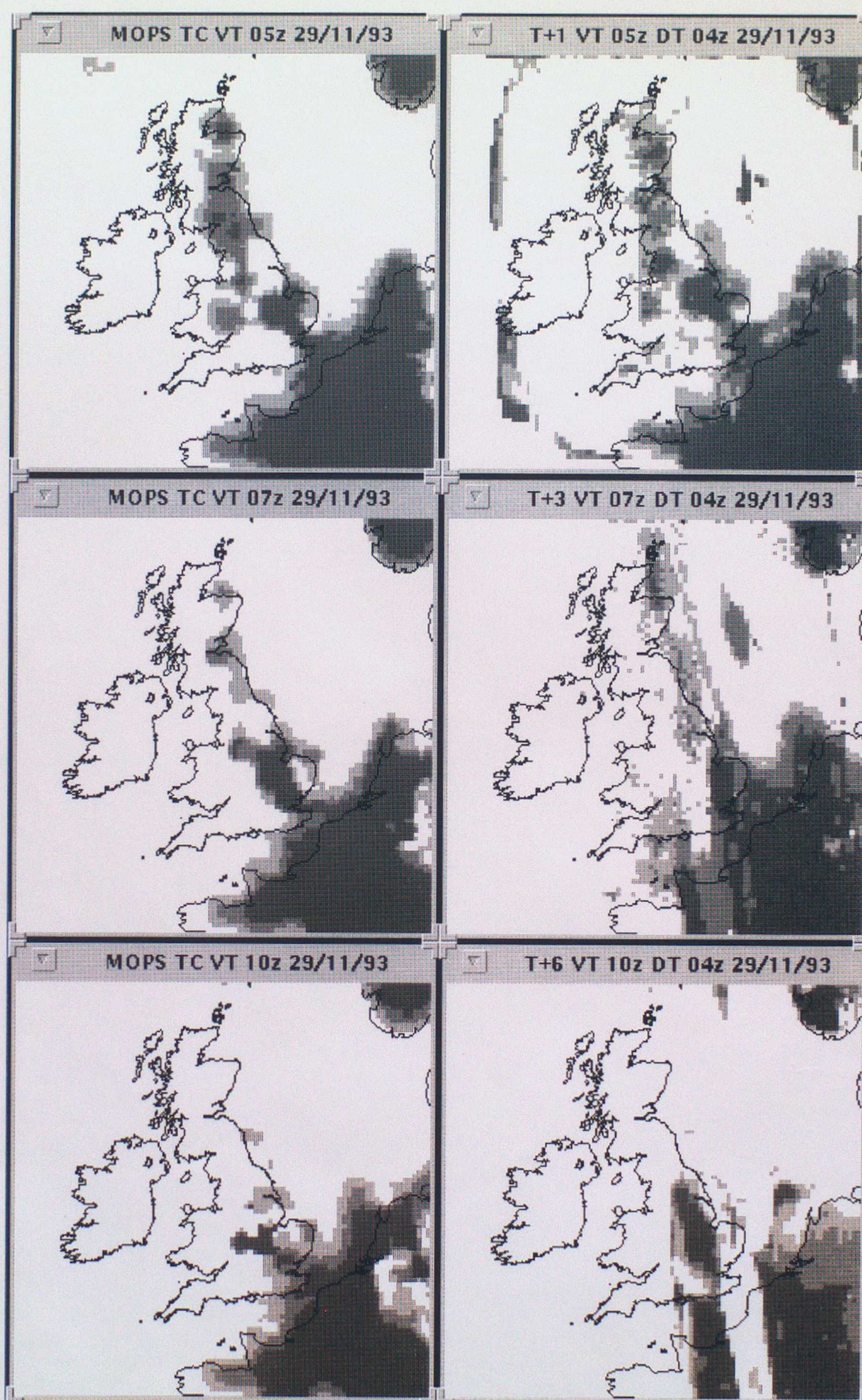
Figure 4. MOPS analyses and corresponding merged cloud amount forecast for total cloud at T+1, T+3 and T+6 from data time 29/11/93 0400 UTC. White = 6/8 - 8/8, light grey 4/8 - <6/8, grey 2/8 - <4/8 and dark grey 0 - <2/8 cover.
