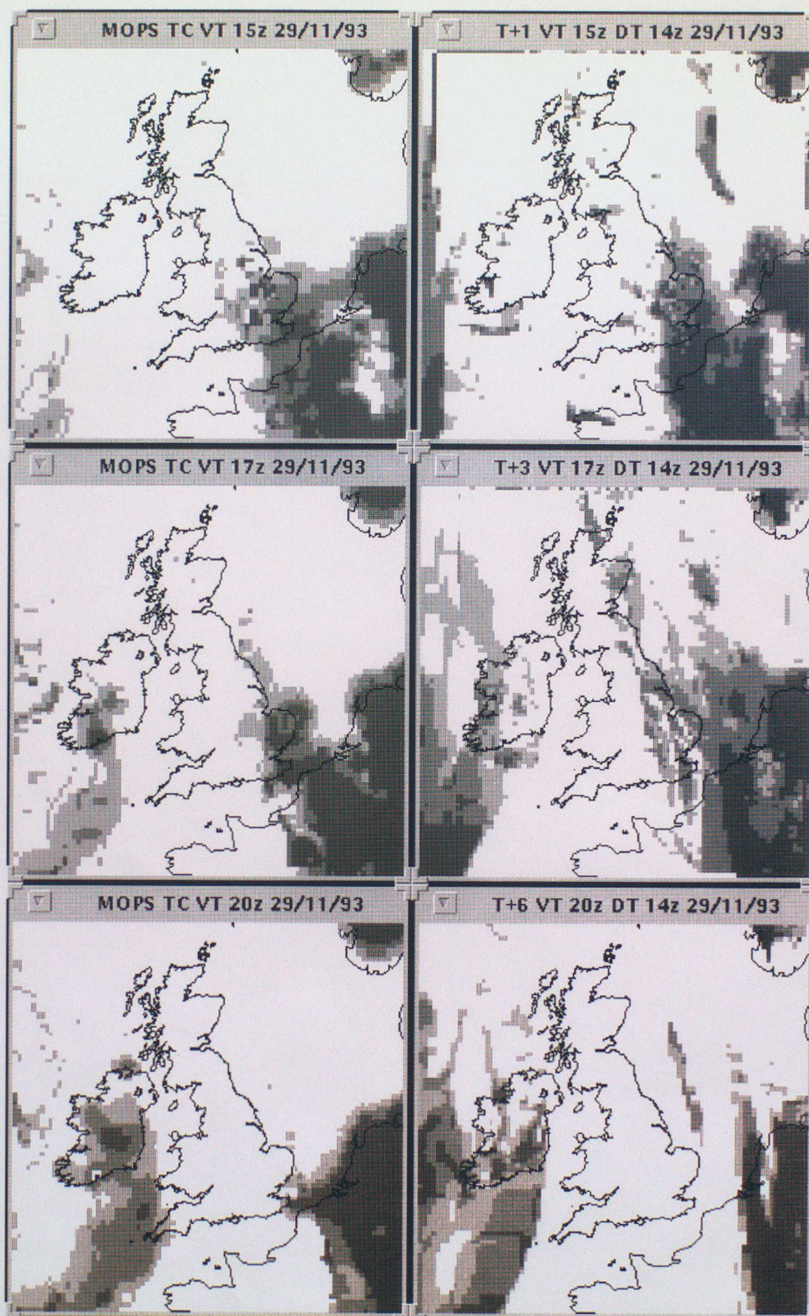
Figure 6. MOPS analyses and corresponding merged cloud amount forecast for total cloud at T+1, T+3 and T+6 from data time 29/11/93 1400 UTC. White = 6/8 - 8/8, light grey 4/8 - <6/8, grey 2/8 - <4/8 and dark grey 0 - <2/8 cover.
