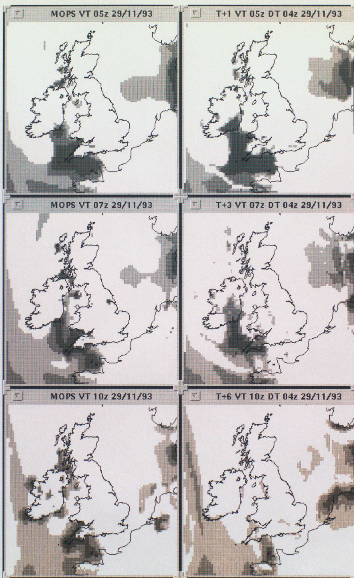
Figure 3. MOPS analyses and corresponding merged cloud amount forecast for low cloud at T+1, T+3 and T+6 from data time 29/11/93 0400 UTC. White = 0 - 2/8, light grey >2/8 - 4/8, grey >4/8 - 6/8 and dark grey >6/8 cover.
