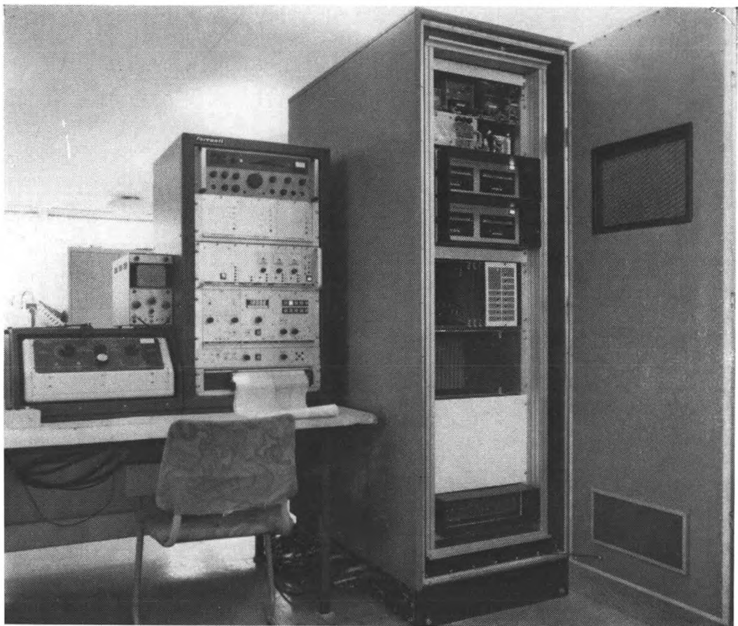
Computer and other ground station equipment for processing signals received from the radiosonde (see page 195)
