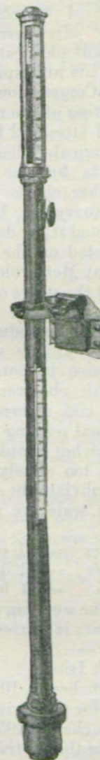
FIG. 3.—KEW PATTERN BAROMETER.
