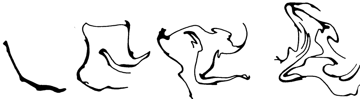
Figure 2. Four stages in the evolution of a patch of dye on the surface of a pan filled with liquid, illustrating enstrophy cascade dispersion. Based upon Welander (1955).
