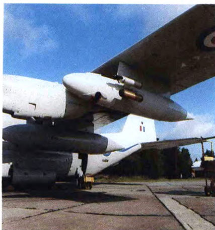
View of the Hercules aircraft showing a pod under the starboard wing carrying cloud physics probes and the multi-channel radiometer.
