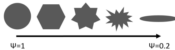
Figure 4: Examples of particle shapes with sphericity between 1 and 0.2.
