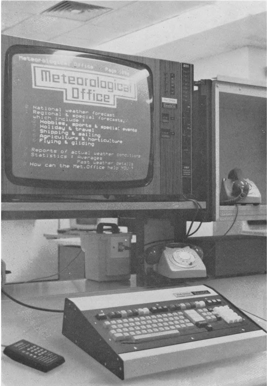
PLATE VI—PRESTEL EDITING TERMINAL SHOWING TELEVISION RECEIVER, EDITING KEYBOARD FOR INPUT AND HAND-HELD KEYPAD FOR SELECTING FRAMES FOR DISPLAY
