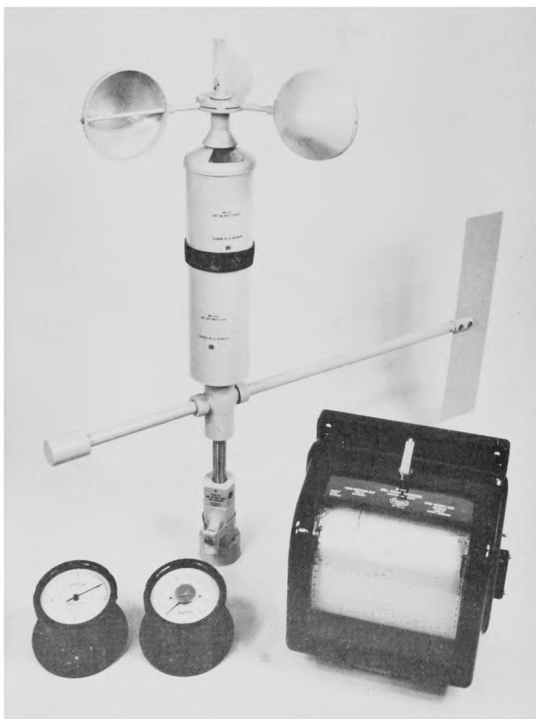
FIGURE 14. Cup generator anemometer Mk 4 with wind vane, dials and recorder
