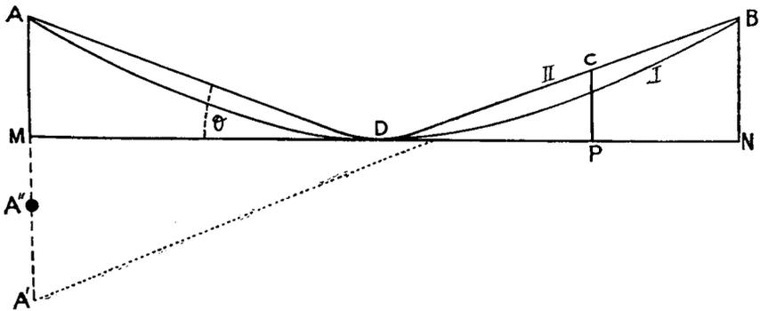
diagram. If, however, the temperature gradient exists only in the layers of air very near to the ground, then the ray will be curved in the neighbourhood of  $D$ , and straight at  $A$  and  $B$ , as (II) in the diagram.
