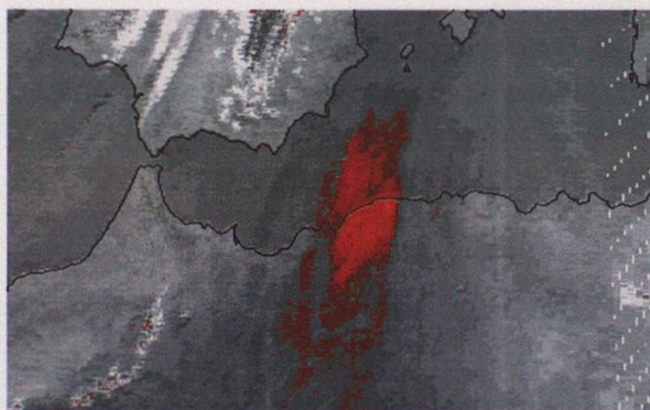
Figure 9. AVHRR ch4-ch5 BTD image over the western part of the Mediterranean Sea on 25 August 2000. Grey to white are positive BTD values, red are negative BTD values. A mineral dust cloud can be seen over the Algerian coast with values of approximately -2 K.
