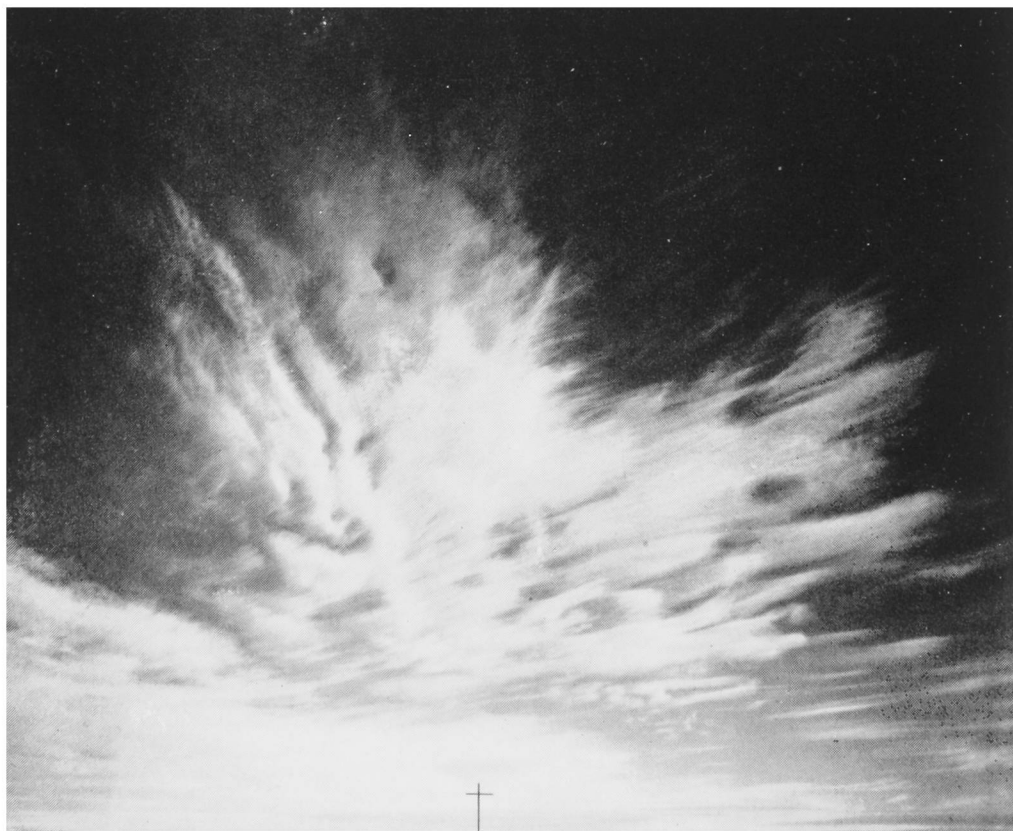
FIG. 3—TWO LOWER BANDS, ONE AT 8,500 FT., ANOTHER AT 6,000 FT., Time: 2239 BRIGHT-BAND CLOUD ECHOES OBSERVED BY RADAR AT SALISBURY, SOUTHERN RHODESIA
