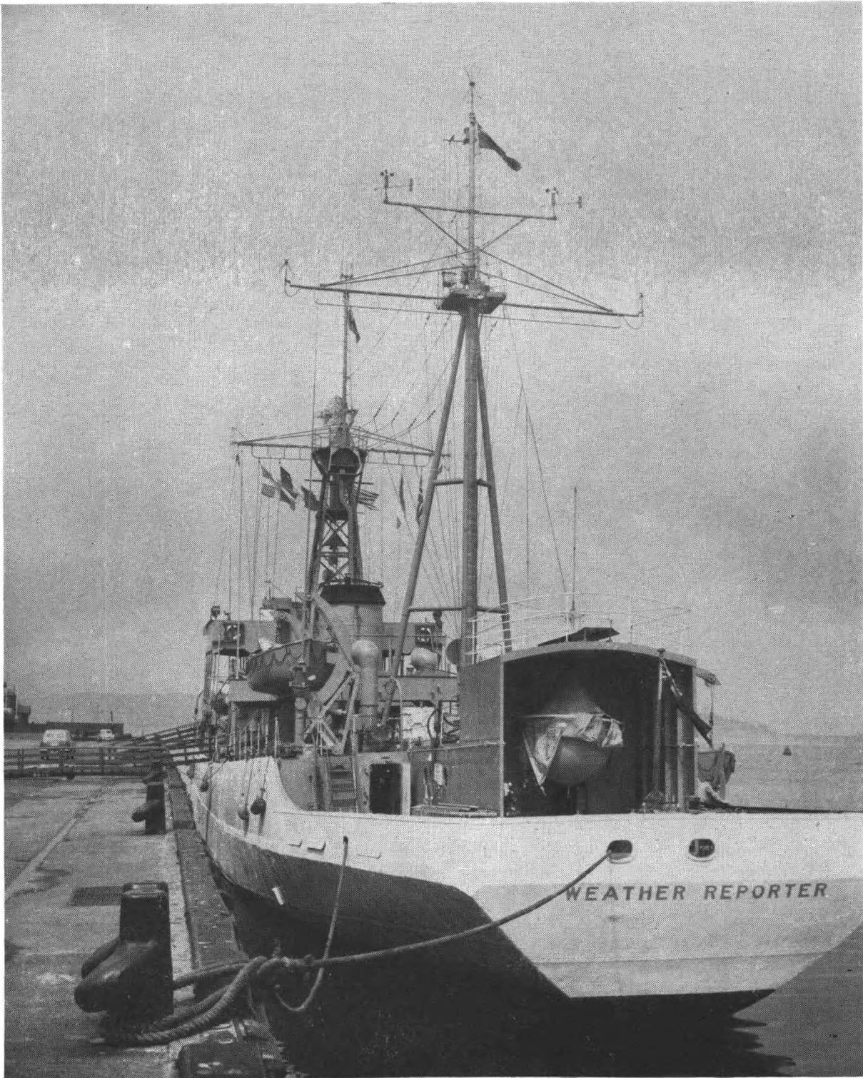
Stern view of Ocean Weather Ship Weather Reporter showing balloon filling shelter and balloon, and anemometers and wind vanes on yard arm. (See p. 18.)
