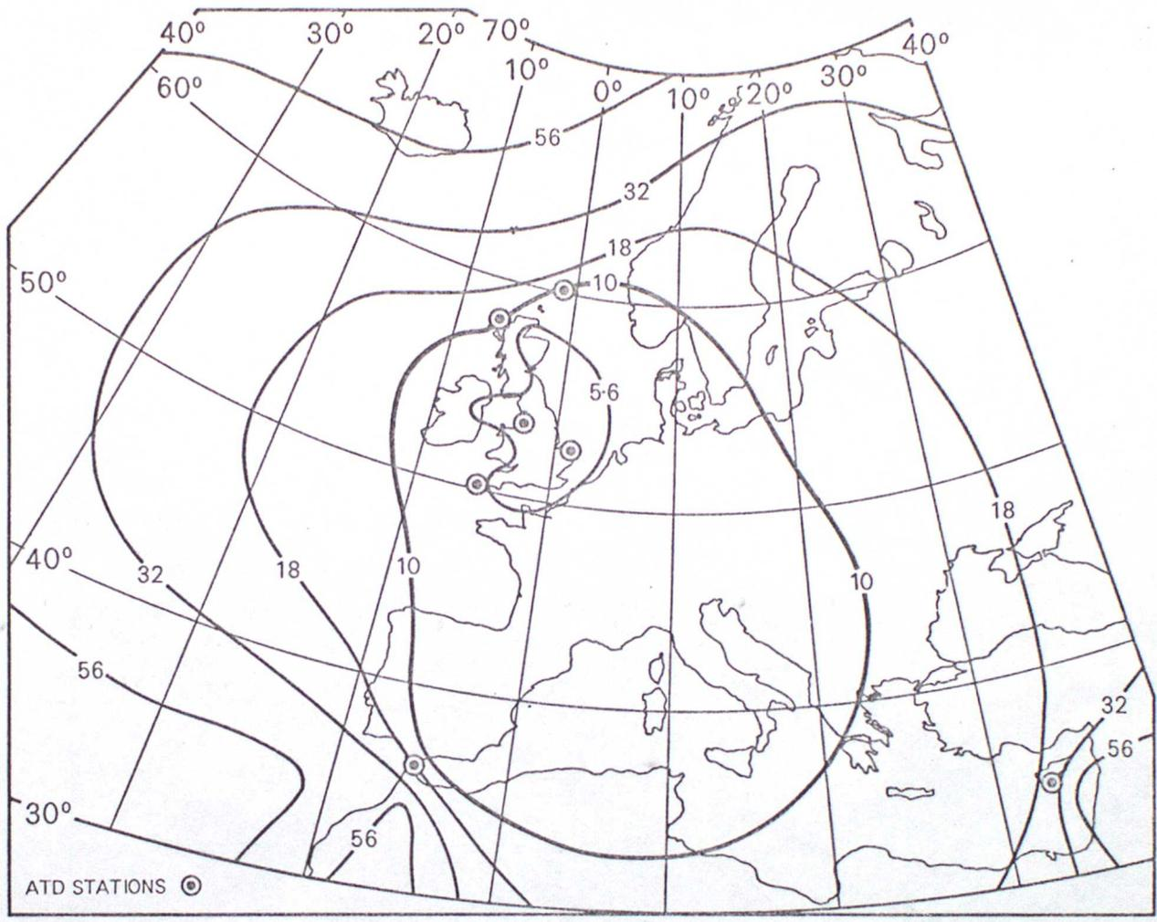
Fig 3: Chart of ATD flash location error (RMS km) assuming 25  $\mu$ s RMS ATD error, for a possible "operational" network.
