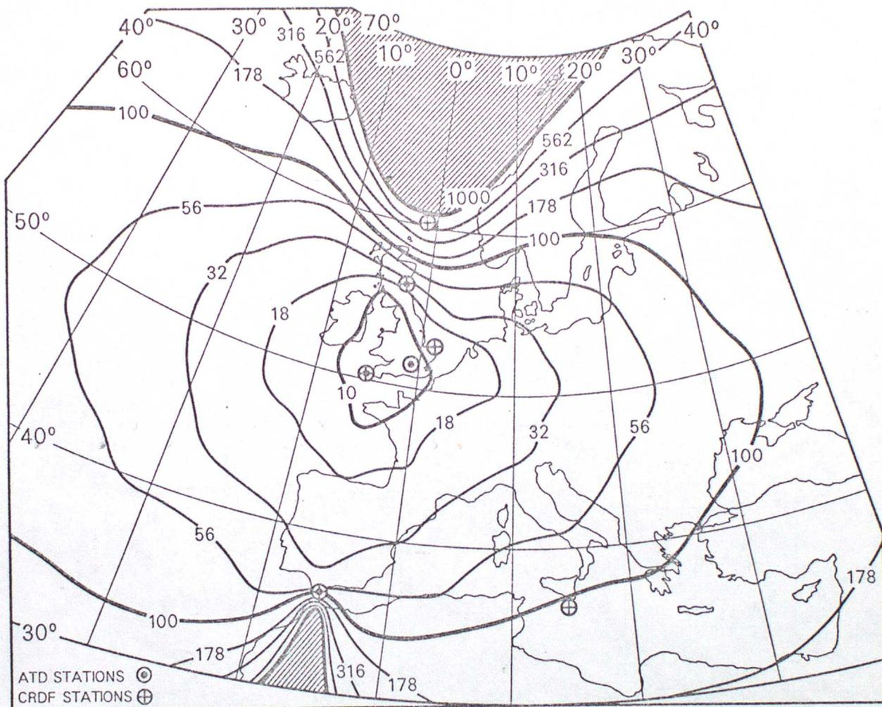
Fig 2: Chart of ATD flash location error (RMS km) assuming 25  $\mu$ s RMS ATD error. The trial deployment of ATD and CRDF stations is shown.
