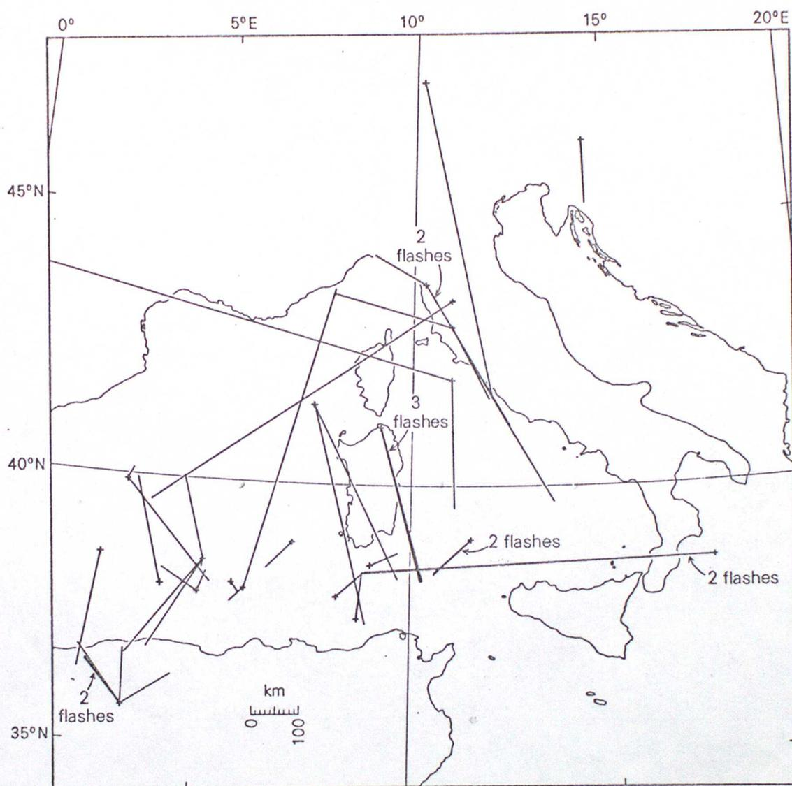
Fig 4: Vectors joining CRDF fixes (+) to the corresponding ATD fixes: Winter conditions.
