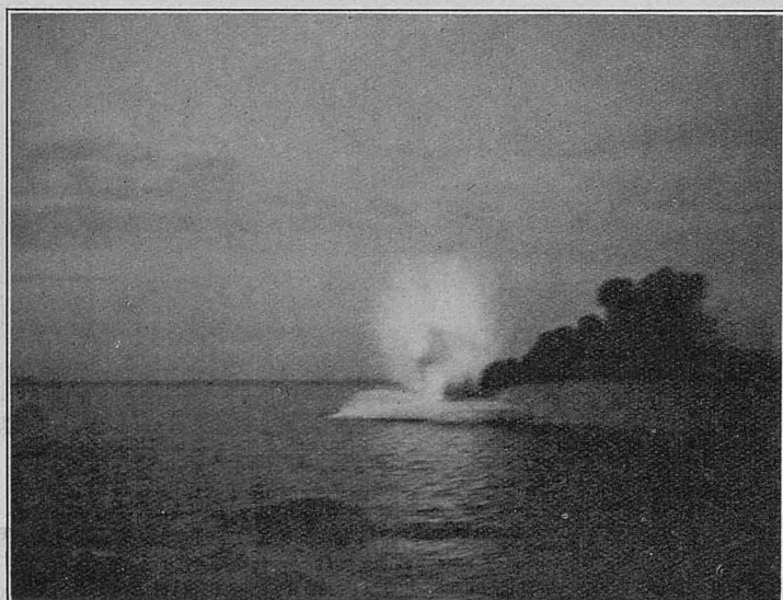
8. Explosion of ice due to 500 pounds of thermit.
